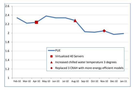
It must be understood that there are many other factors which may impact PUE. There will always be tradeoffs between availability and energy efficiency. Redundancy, for example, will increase PUE. Data center equipment – from cooling equipment to UPSs to server power supplies – will run more efficiently when more heavily loaded.
