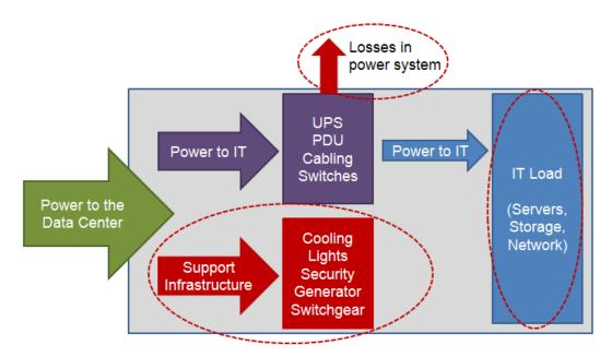
"Reductions in energy consumption at the IT equipment level have the greatest impact on overall consumption because they cascade across all supporting systems".
